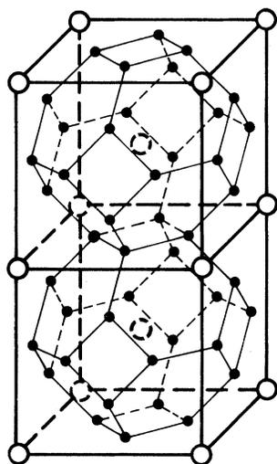
FIG. 3. Tetrahedral interstitial positions in a bcc lattice.
