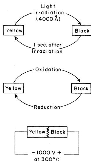
FIG. 1. Processes that produce reversible color changes in  $\text{SrTiO}_3$ .
