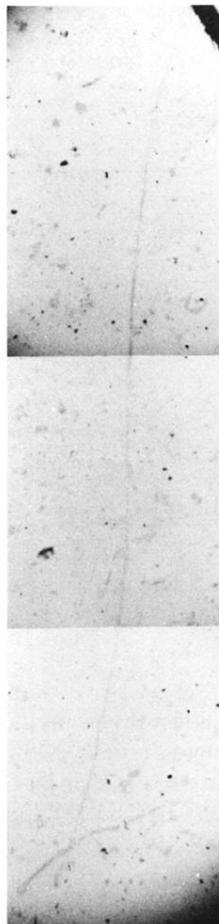
FIG. 3. Spots are projections of  $\alpha$ -particle tracks on the surface of the  $\text{SrTiO}_3$  crystal. Most of the  $\alpha$  particles emitted during the decay of uranium are stopped in the oxide layer. The range of these  $\alpha$  particles in the oxide is  $\sim 10\mu\text{m}$ . The long track is apparently due to a cosmic-ray particle being slowed down and reacting with a nucleus in the oxide layer. The total length of the track is 4.6 mm.
