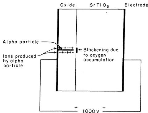
FIG. 2. Experimental arrangement used in detection of radiation.  $\alpha$  particles release positive oxygen ions in the uranium-oxide layer. The positive oxygen ions are attracted to  $\text{SrTiO}_3$  and oxygen accumulation produces color changes on the surface of the crystal. The depth of the blackening is too small to measure. Thickness of the  $\text{SrTiO}_3$  crystal is 2 mm and the thickness of the oxide layer is  $\sim 0.1$  mm.
