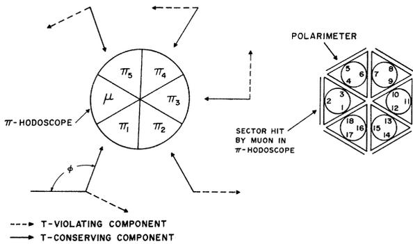
FIG. 2. (a) The five inequivalent  $K_L^0 \rightarrow \pi^- \mu^+ \nu_\mu$  event types and schematic illustration of  $T$ -invariant and  $T$ -noninvariant components of  $\mu^+$  polarization transverse to the  $K_L^0$  beam axis. (b)  $e^+$  counters in the polarimeter.
