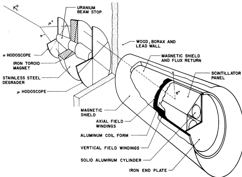
FIG. 1. Perspective view of the experimental apparatus. Drawing not to scale; see text for approximate dimensions.
