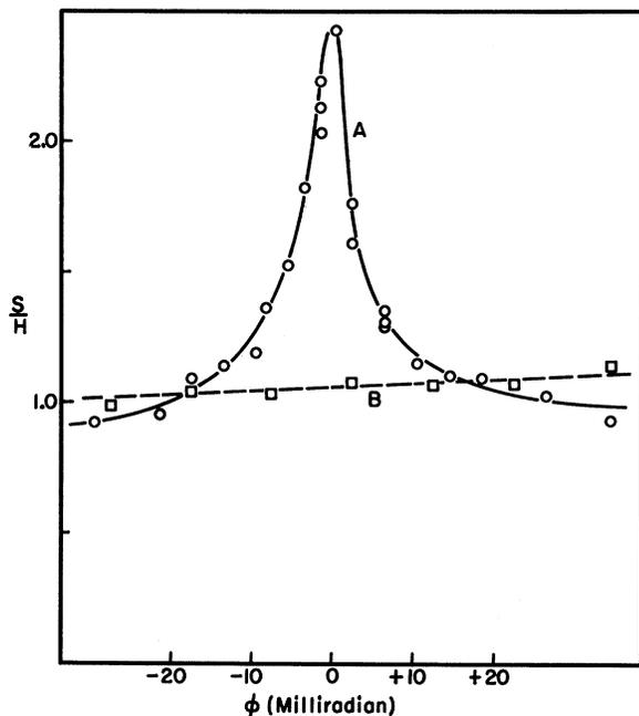
FIG. 1. The relative change measured in the ratio of soft quanta to hard quanta ( $S/H$ ) as the crystal was turned through  $\phi$  with  $\psi \approx 0$  (curve A) and  $\psi \approx 20$  milliradians (curve B).
