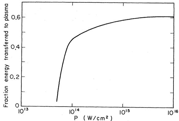
FIG. 2. Fractional energy transfer as a function of laser power density.
