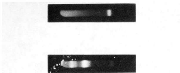
FIG. 1. Flash x-ray diffraction records of BN. The top record was obtained before shock-wave compression, and exhibits only the 004 Cu K\beta line. The bottom record was taken at the instant the shock wave emerged from the front of the sample.
