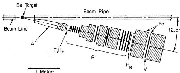
FIG. 1. Schematic diagram of the detector. Each gap in the iron contains a single  $R$  or  $V$  counter, as indicated. Lead shielding between the detector and the photon beam is not shown. The beam enters from the left.
