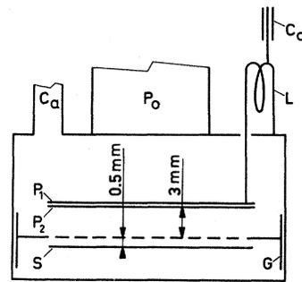
FIG. 2. Schematic representation of resonant circuit with sample chamber.  $C_0$ , coaxial cable carrying 200 MHz.  $C_a$ ,  $^4\text{He}$ -filled capillary.  $P_0$ ,  $^3\text{He}$  pot.  $P_1$ ,  $P_2$ , G, and S, electrodes (see text). L, self-inductance and autotransformer.
