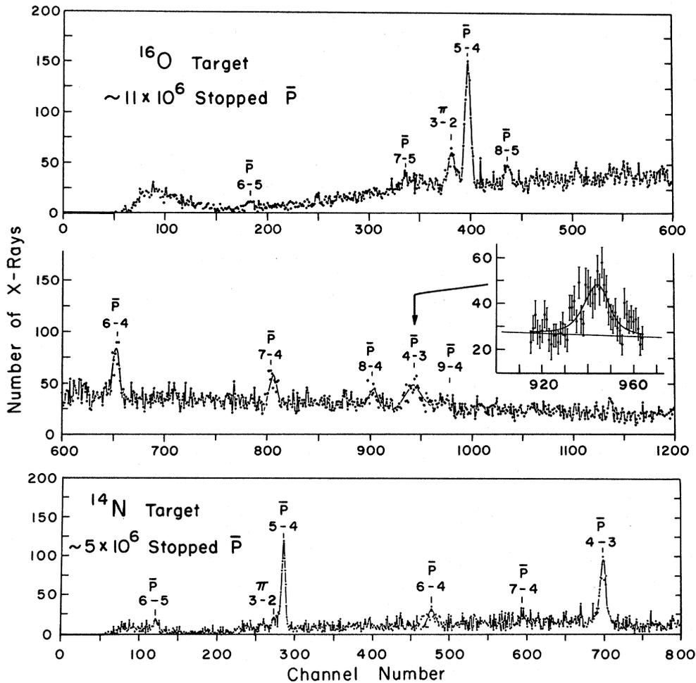
FIG. 1. X-ray spectra from antiprotonic atoms of  $^{16}\text{O}$  and  $^{14}\text{N}$ . The dispersion was 72.42 eV per channel. The energy  $E$  in terms of channel number  $n$  is given by  $E = (0.07242n + 5.107)$  keV.
