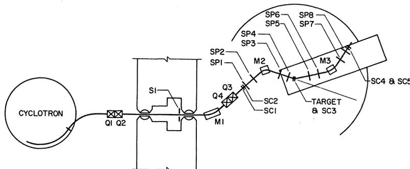
FIG. 1. Experimental setup.  $SC_1$ – $SC_5$  are scintillation counters,  $SP_1$ – $SP_8$  are sonic spark chambers,  $M_1$ – $M_3$  are bending magnets,  $Q_1$ – $Q_4$  are quadrupole magnets, and  $S_1$  is a beam-defining slit.
