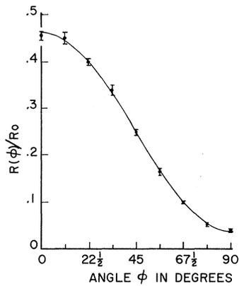
FIG. 3. Coincidence rate with angle  $\phi$  between the polarizers, divided by the rate with both polarizers removed, plotted versus the angle  $\phi$ . The solid line is the prediction by quantum mechanics, calculated using the measured efficiencies of the polarizers and solid angles of the experiment.
