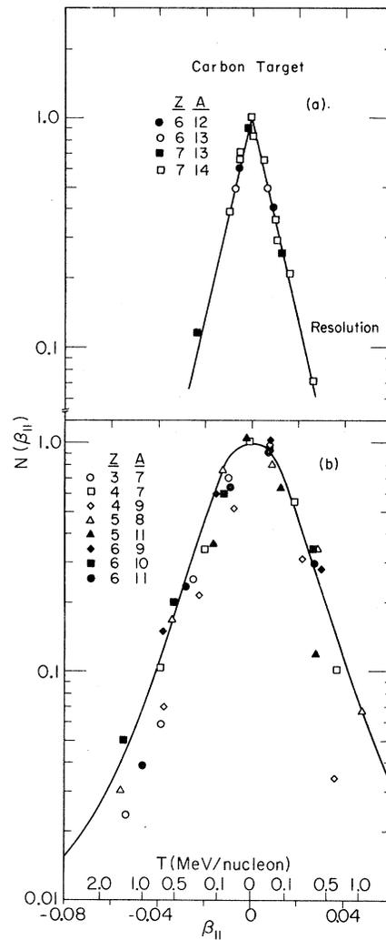
FIG. 2. Distribution of longitudinal velocities and energies/nucleon of  $^{14}\text{N}$  fragmentation products in the projectile frame. (a) Nuclei with mass numbers  $12 \leq A \leq 14$ . The resolution function is the apparent  $N(\beta_{\parallel})$  for the monoenergetic  $^{14}\text{N}$  beam. (b) Nuclei with mass numbers  $7 \leq A \leq 11$ . Solid curve drawn through data represents a composite of the  $\beta_{\parallel}$  spectra for these nuclei.
