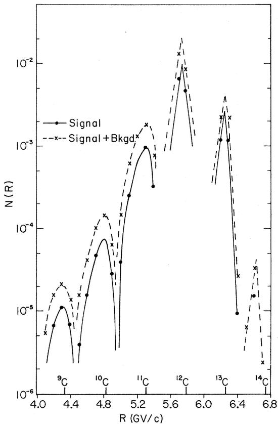
FIG. 1. Rigidity spectrum of carbon isotopes produced by the fragmentation of 29-GeV  $^{14}\text{N}$  nuclei. The differential intensity has been normalized to give the observed count-rate per incident  $^{14}\text{N}$  beam particle on the carbon target ( $4.36 \text{ g cm}^{-2}$ ).
