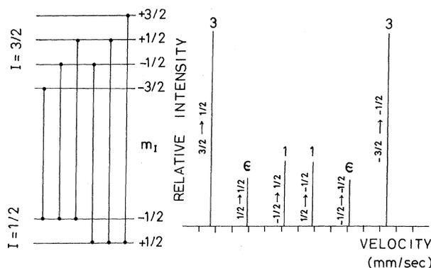
FIG. 2. Energy-level diagram and magnetic hyperfine spectrum of the Mössbauer transitions in <sup>57</sup>Fe. The energy levels are drawn for an isolated iron nucleus in an external field. The relative intensity indicated by  $\epsilon$  depends on the orientation of the field.
