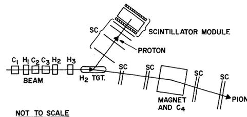
FIG. 1. Spectrometer system.  $C_1$ - $C_4$ , threshold Cherenkov counters;  $H_1$ - $H_3$ , beam hodoscopes. Spark chambers, denoted by SC. Beam magnets, trigger and veto counters, and scintillators that measure charge multiplicity, not shown.
