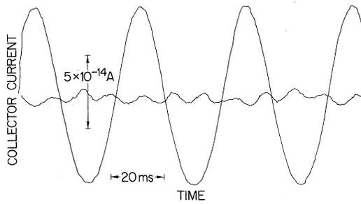
FIG. 2. Typical current signal received at the collector. The trace in the middle is obtained when the vortex beam is off but the ac is on. The sine wave is obtained for a 20-eV beam,  $V_{ac} = 0.2$  V and  $f = 25.5$  Hz.
