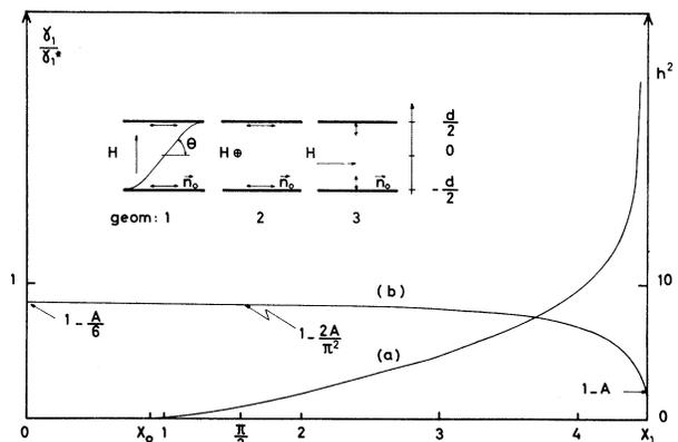
FIG. 1. MBBA in geometry 3: curve *a*, the wave vector of the distortion  $k = 2d^{-1}X$  as a function of the reduced field  $h = H/H_c$ ; curve *b*, the normalized effective viscosity  $\gamma_1^*(X)$ . It is practically a constant for the fields values used in this experiment. The inset refers to the three geometries discussed.
