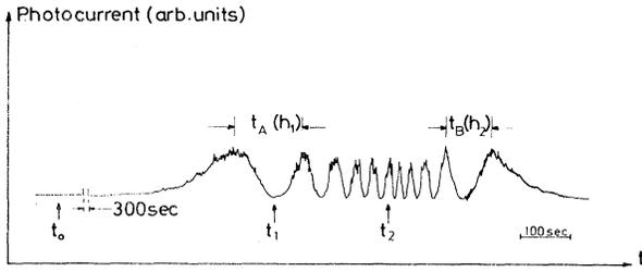
FIG. 2. Dynamical behavior when a field  $h_1$  is applied at time  $t_0$  (or is suddenly decreased to  $h_2$  at time  $t_2$ ), characterized by the time difference of the first two successive conoscopic fringes  $t_A(h_1)$  [ $t_B(h_2)$ ].
