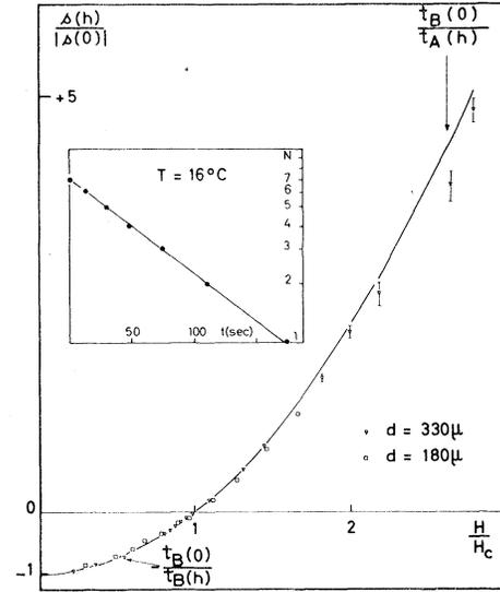
FIG. 3. Time constant of the distortion, as measured by  $s^{-1}(h)$ , normalized to the value for  $h = 0$ , which follows the  $h^2 - 1$  law predicted accurately by the theory. Note in particular the divergence of the time constant as  $|1 - h|^{-1}$  at  $H_c$ . The exponential relaxation of the distortion for  $h_2 = 0$ , close to the equilibrium, is followed by the indexed number of fringes  $N(t)$  (inset) and is used to measure  $\gamma_1^*$ .
