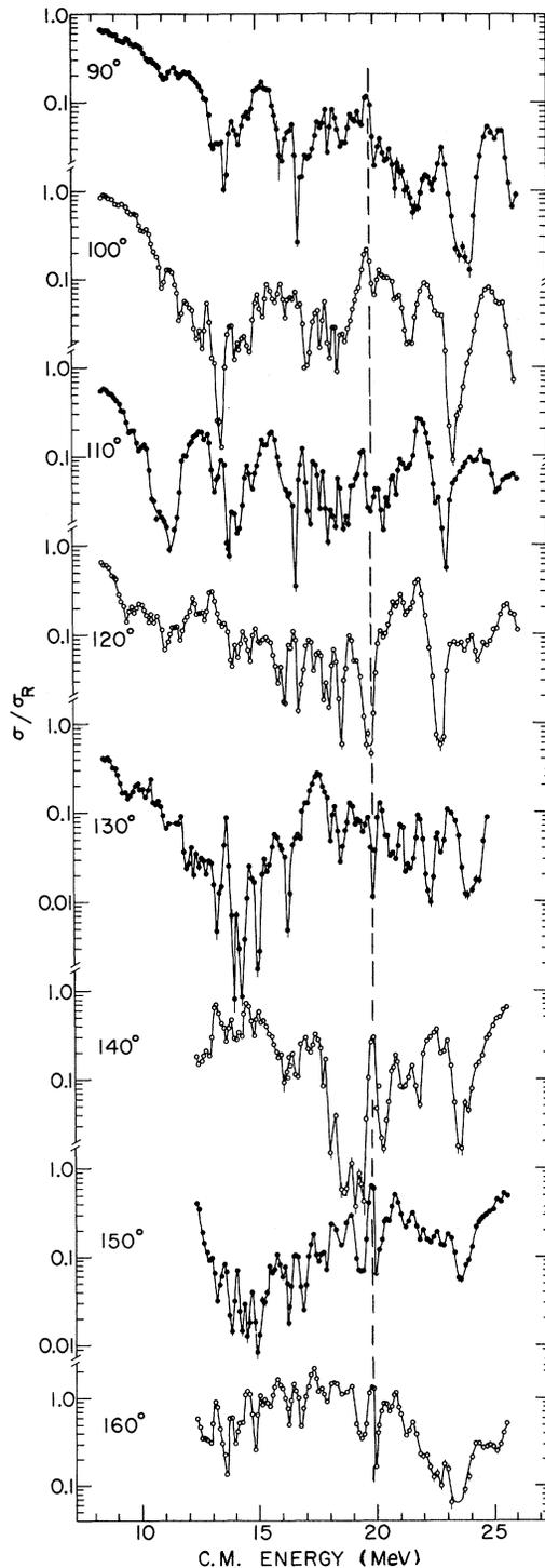
FIG. 1. Elastic-scattering excitation functions plotted as ratios of differential cross sections to Rutherford-scattering cross sections. The dashed vertical line indicates the position of the 19.7-MeV anomaly.
