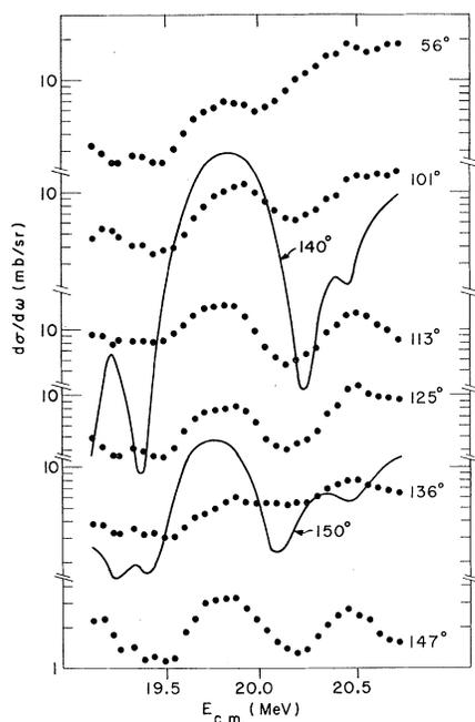
FIG. 3.  $^{12}\text{C}(^{16}\text{O}, ^{16}\text{O}^*)^{12}\text{C}$  inelastic-scattering cross sections for transitions to the unresolved  $0^+$ ,  $3^-$  states at 6.1 MeV in  $^{16}\text{O}$ , as measured with a thin target. Solid curves, unnormalized elastic scattering excitation functions at  $140^\circ$  and  $150^\circ$ , which also have been measured with a thin target.
