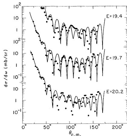
FIG. 4. Elastic-scattering angular distributions on and off resonance. Solid curves, calculated with an optical model plus a Breit-Wigner resonance term for  $L=14$ .
