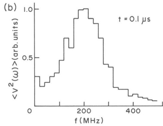
FIG. 2. (a) Example of observed fluctuations. Scale, 5 nsec/cm. (b) Power spectrum of the fluctuation averaged over eight oscillograms taken under the same conditions:  $\bar{n} = 2 \times 10^{17} \text{ m}^{-3}$ ,  $V_c = 8.5 \text{ kV}$ ,  $B = 1.5 \text{ kG}$ .
