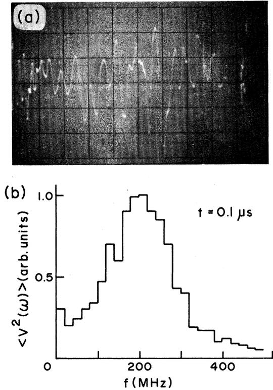
FIG. 2. (a) Example of observed fluctuations. Scale, 5 nsec/cm. (b) Power spectrum of the fluctuation averaged over eight oscillograms taken under the same conditions:  $\bar{n} = 2 \times 10^{17} \text{ m}^{-3}$ ,  $V_c = 8.5 \text{ kV}$ ,  $B = 1.5 \text{ kG}$ .
