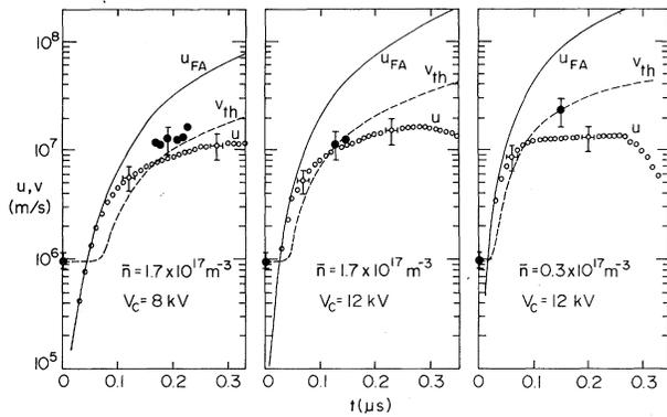
FIG. 1. Electron drift and thermal velocities. Open circles, measured average drift velocity  $u$ ; solid lines, velocity for free acceleration,  $u_{FA}$ ; closed circles, measured thermal velocity  $(\kappa T_e/m)^{1/2}$ ; dashed lines, thermal velocity calculated from energy balance,  $v_{th}$ . For all three cases the argon gas pressure  $p = 0.3$  mTorr and  $\vec{B} = 1.0$  kG.
