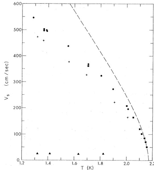
FIG. 3. Superfluid velocity as a function of temperature at a pressure head of 35  $\mu\text{m}$  of He, for several orifices. Circles and squares: orifice C on two dates three days apart; crosses: orifice D; triangles: orifice No. 1, without rouge plugs. The dashed line is the function  $\rho_s(T)/\rho T$  with arbitrary normalization.
