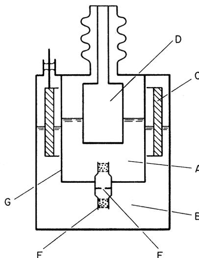
FIG. 1. Schematic diagram of the apparatus: A, inner helium reservoir; B, outer reservoir; C, capacitor; D, plunger; E, pinhole; F, rouge plug; G, oxygen-free high-conductivity copper wall.
