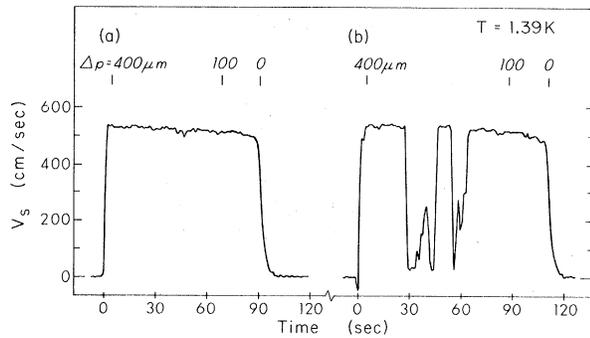
FIG. 2. Data for two runs, showing superfluid velocity as a function of time during decay of an initial pressure head. The head in micrometers of He is indicated at several points.
