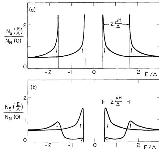
FIG. 1. Theoretical density of states for a superconductor in a magnetic field  $H = 0.6\Delta/\mu$ . (a) With  $b = 0$ ,  $N_S(E/\Delta)$  splits into two BCS-like curves, one for each spin direction shifted by  $\pm \mu H$ . (b) With some spin-orbit scattering,  $b = 0.2$ , the spin states are mixed with some spin-up states found near the energy of the spin-down peak.
