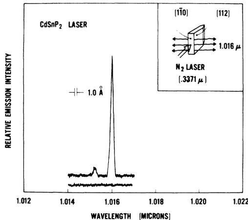
FIG. 2. Laser emission spectra at  $80^\circ\text{K}$  measured, respectively, slightly below and 15% above threshold of  $\sim 50 \text{ kW/cm}^2$ . As shown in the inset, the nitrogen laser was incident onto a cleaved  $[1\bar{1}0]$  face, and the natural  $[112]$  faces formed the Fabry-Perot resonator. The mode spacing agrees with cavity length ( $110 \mu\text{m}$ ) and  $n - \lambda_0 \partial n / \partial \lambda = 6.3$  (Ref. 10).
