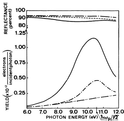
FIG. 1. Reflectance and photoyield measurements on Al. Solid curves, measurements taken on one of the slightly roughened films with coupling to surface waves appreciable; dot-dashed lines, reflectance and photoyield measurements on the smoothest Al films that we made. The dashed line is the scattered-light-induced reflectance drop in the rougher film (Ref. 17). The double-dot-dashed curve is our estimate of the ideally smooth-surface photoyield, i.e., no surface-wave contribution.
