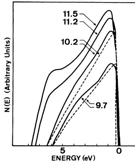
FIG. 3. Electron distribution curves for excitation energies just above and just below the Al surface plasma frequency (10.55 eV). Dashed curves are theoretical EDC's calculated in the surface photoeffect theory (Refs. 1, 11). EDC's were plotted for comparison of shapes and are *not* normalized to photoyield.
