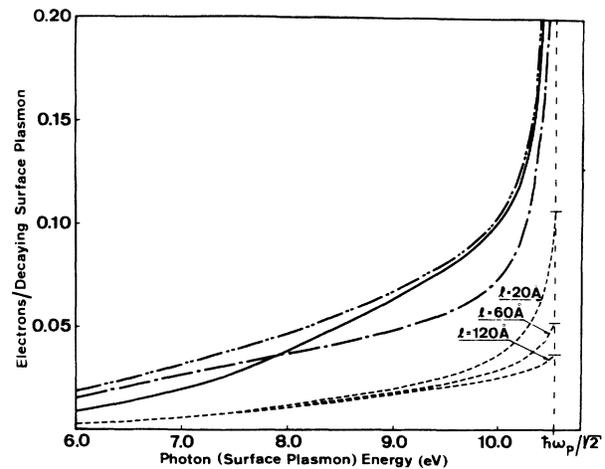
FIG. 2. Experimentally determined and calculated electrons per decaying surface plasmon (surface wave) in Al. Solid curve, experiment; dashed curve, surface-wave decay in the volume photoeffect theory; dot-dashed curve, surface-wave decay in the surface theory; double-dot-dashed curve, the sum of the volume and surface theories.
