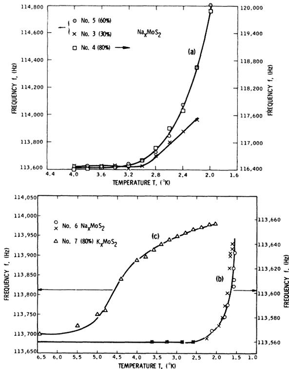
FIG. 2. Onset of the superconducting transition in (a) intercalated natural crystals of molybdenite, (b) intercalated synthetic crystals of MoS<sub>2</sub>, and (c) intercalated purified natural ore. The percentage of the sample intercalated is shown in parentheses. (Preliminary chemical analysis of sample No. 6 indicates that it is 65% intercalated.)
