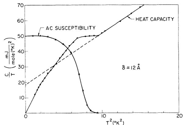
FIG. 2. The measured heat capacity and magnetic susceptibility of  $\text{TaS}_2(\text{aniline})_{0.75}$  from 1 to 4.5°K. The specific-heat anomaly appears smaller in this sample than in  $\text{TaS}_2(\text{pyridine})_{1/2}$  for two reasons: The contribution to the background is larger because there is more organic material per  $\text{TaS}_2$  and the normal-state extrapolation (shown as dashed line) is not valid for this sample (see text). In fact the two anomalies are quite similar.
