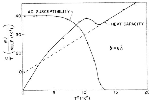
FIG. 1. The measured heat capacity and magnetic susceptibility of  $\text{TaS}_2(\text{pyridine})_{1/2}$  from 1 to 4.5°K. The normal-state extrapolation is shown as a dashed line.
