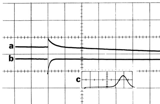
FIG. 2. Oscilloscope traces. (a) Undeflected beam current in Faraday cup (2 V, 100  $\mu$ sec per large division); (b) integrated photodiode current (0.2 V, 100  $\mu$ sec); (c) corresponding instantaneous photodiode current (19.8 V, 10 nsec).
