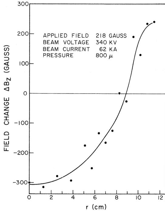
FIG. 4. Radial dependence of field changes  $\Delta B_z$ .
