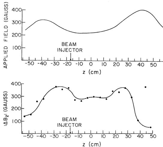
FIG. 5. Applied field  $B_0$  and field changes  $|\Delta B_z|$  on axis.
