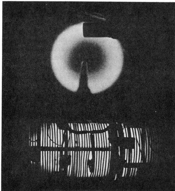
FIG. 2. Optical recordings of *E* layer (top: axially; bottom: from side).
