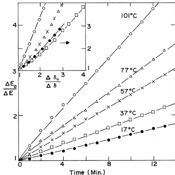
FIG. 1. The normalized inverse modulus defect plotted as a function of time for the indicated temperatures. The sample material was copper (99.9%) and the production rate was  $2.5 \times 10^{10}$  defects/sec  $\text{cm}^3$ . The inset shows a plot of the normalized inverse modulus defect  $Y^{-1}$  versus the normalized inverse decrement  $Z^{-1}$ .
