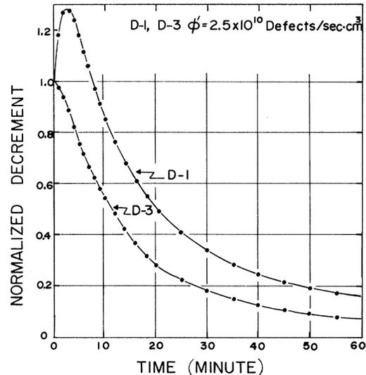
FIG. 3. The decrement normalized to its value at time  $t=0$  and plotted as a function of time of irradiation at 290°K. The sample temperature during irradiation, the high-temperature annealing temperature, and the initial decrement are, for D-1,  $T_{\text{irr}}=290^\circ\text{K}$ ,  $T_{\text{anneal}}=1003^\circ\text{K}$ ,  $\delta_0=2.44 \times 10^{-3}$ ; for D-3,  $T_{\text{irr}}=290^\circ\text{K}$ ,  $T_{\text{anneal}}=1053^\circ\text{K}$ ,  $\delta_0=10.7 \times 10^{-3}$ .
