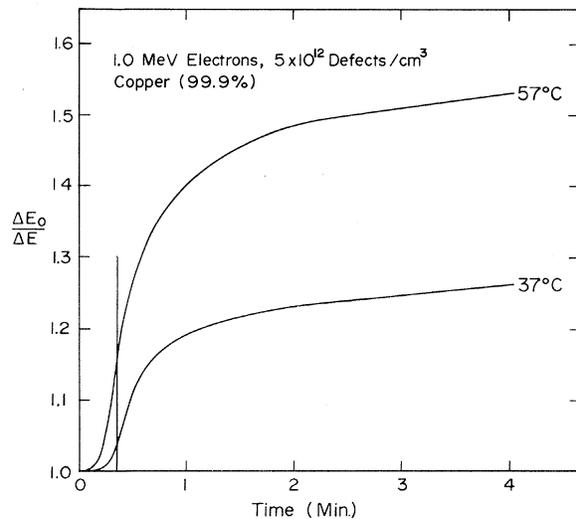
FIG. 2. The normalized inverse modulus defect plotted as a function of time for the indicated temperatures. The vertical line at 22 sec indicates the end of the pulse irradiation.
