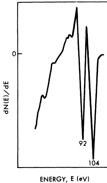
FIG. 1. Auger electron spectrum for clean polycrystalline beryllium.
