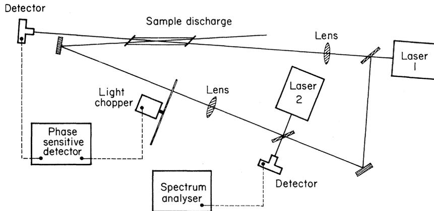
FIG. 1. Experimental setup. When measuring the interaction signal, the beam from laser 2 is blocked off.
