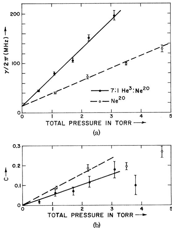
FIG. 3. Experimental results for (a) linewidth  $\gamma$  and (b) cross-relaxation parameter  $C$  versus pressure for a 7:1 mixture of He<sup>3</sup>:Ne<sup>20</sup> and for pure Ne<sup>20</sup> discharges. The error bars denote two standard deviations in the parameters determined by a least-squares curve-fitting computer program.
