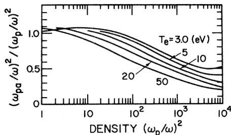
FIG. 1. Calculation of  $(\omega_{pa}/\omega)^2/(\omega_p/\omega)^2$  at  $\omega_c/\omega = 0.95$  for various values of  $T_e$  (eV).
