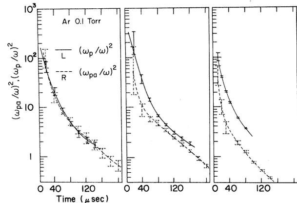
FIG. 2. Electron density decay measured by the  $R$  and  $L$  waves; (a)  $\omega_c/\omega = 0.5$ , (b)  $\omega_c/\omega = 0.8$ , and (c)  $\omega_c/\omega = 0.95$ .
