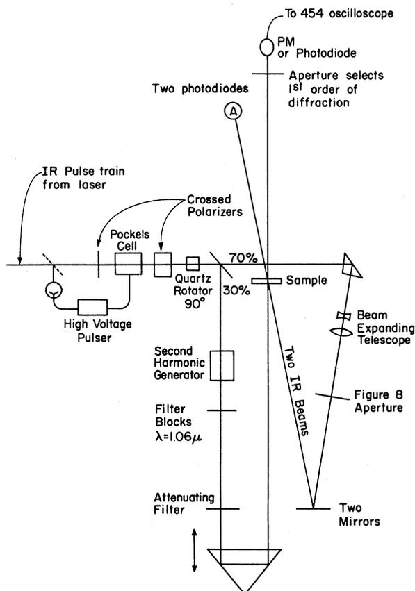
FIG. 1. Arrangement of the apparatus. At the point marked A are two photodiodes, one above the other. The upper one is connected to a 519 oscilloscope and monitors the IR pulse train by looking at the lower of the two transmitted beams. The lower diode is positioned in the first scattered IR beam below the two transmitted beams, and can be connected to the 454 oscilloscope to study the IR scattering.
