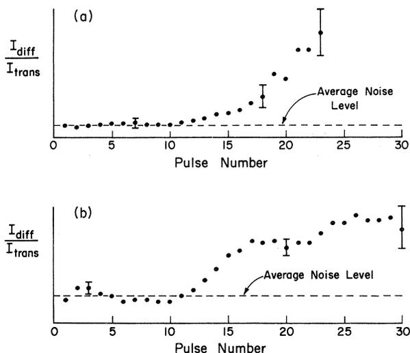
FIG. 2. Typical ratios of diffracted light to transmitted IR light for the cupric nitrate sample (arbitrary units). Each graph is taken from a single-pulse train recorded simultaneously with two oscilloscopes. (a) Shows diffracted IR light; (b) shows diffracted green. The average noise level is the ratio observed when one of the two IR beams aimed at the sample is blocked.
