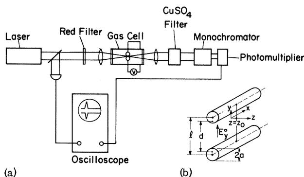
FIG. 1. (a) Schematic diagram of the apparatus. (b) Electrode geometry.
