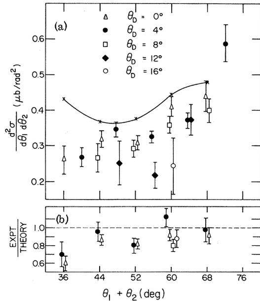
FIG. 3. (a) Cross sections defined by Eq. (3) as a function of  $\theta_S$  and  $\theta_D$ . (b) The ratios of experimental to theoretical cross sections for symmetric polar angles. Closed circles represent coplanar cross sections, and triangles double differential cross sections. Recent Oak Ridge results (Ref. 4) are shown as an open circle and square, respectively.
