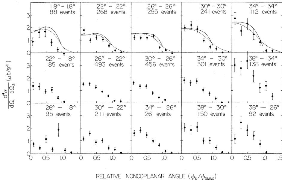
FIG. 2. Cross sections defined by Eq. (2) for various polar-angle combinations, as a function of  $\varphi_r$ . The dashed curve represents theoretical cross sections after the experimental angular resolution (always equal to about  $\pm 0.2$  in  $\varphi_r$ ) has been folded in.
