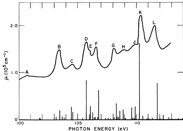
FIG. 2. Comparison of  $\mu$ , the measured absorption coefficient for Ce in the region of the  $N_{IV,V}$  edge from Ref. 2, with the calculated relative positions and line strengths of  $4d^{10}4f^2 F_{5/2} \rightarrow 4d^9 4f^2$  transitions. Additional line positions corresponding to prominent peaks in the ionization region are shown in Table I.
