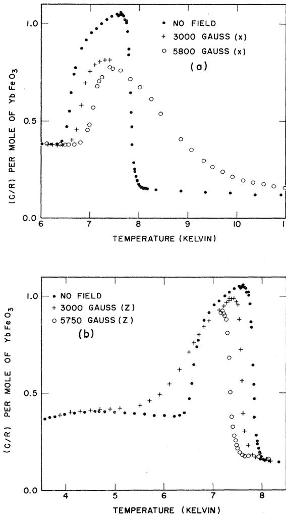
Fig. 2. Specific heat of  $\text{YbFeO}_3$  in applied magnetic fields. (a) Specific heat with field applied along the  $x$  axis. (b) Specific heat with field along the  $z$  axis. The data scatter at the peak of the "no-field" curve reflects differences between different runs. For each run the data fall on a smoother curve.
