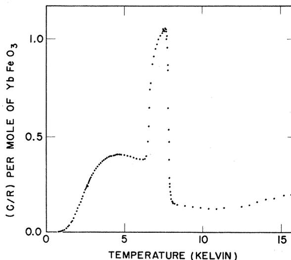
Fig. 1. Specific heat of  $\text{YbFeO}_3$  from 0.4 to 15 K. Data from three different runs are included.
