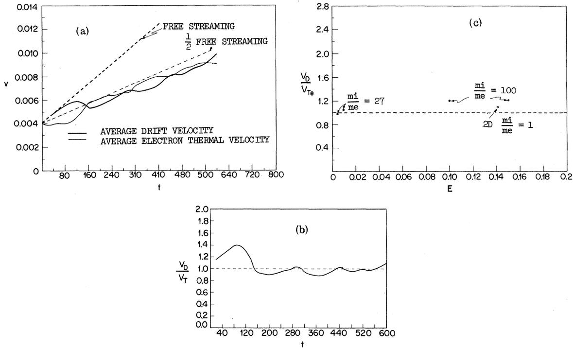
FIG. 3. One- and two-dimensional results on anomalous resistance. (a) Drift and thermal velocity for a typical one-dimensional run follow the same behavior as two-dimensional calculation. (b)  $V_D/V_{Te}$  oscillated slightly about unity. (c) The average value of  $V_D/V_{Te}$ .
