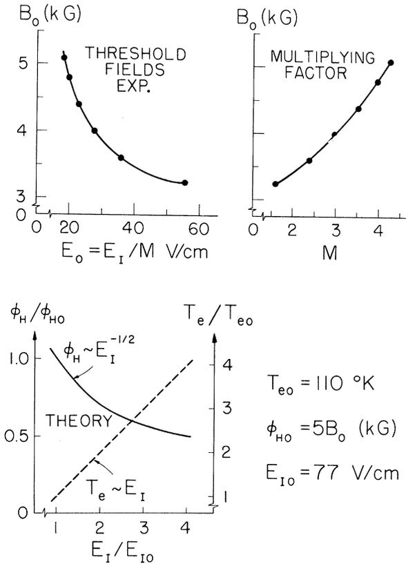
FIG. 2. Experimental values of electric and magnetic field required to maintain a constant threshold (minimum detectable) emission level equivalent to that of a thermal source of  $(0.5-1.0) \times 10^3$  °K at 9.0 GHz. The theoretical model for which  $T_e \sim E_I$  and  $\phi_H \sim E_I^{-1/2}$  requires that the multiplying factor  $M$  vary with  $B_0$  as shown in order to obtain an exact fit to the experimental threshold fields and emission level.
