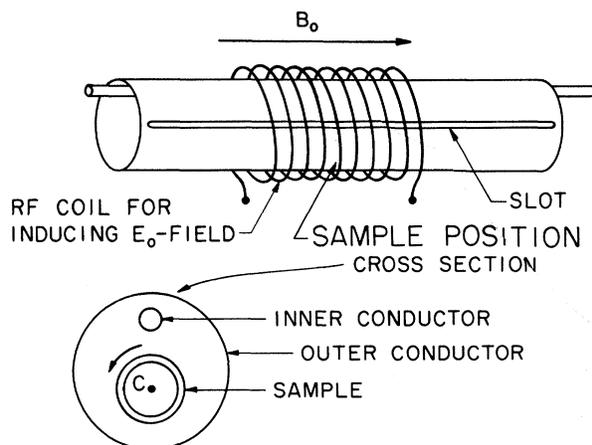
FIG. 1. Schematic representation of the eccentric transmission line and sample system. Microwave tuning is adjusted with a sliding short at one end of the line. A static magnetic field  $B_0$  is applied as shown. The structure is immersed in liquid nitrogen.
