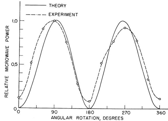
FIG. 3. Relative microwave power measured as a function of sample rotation compared with computations which assumed that the microwave current distribution around the loop sample was produced by a localized source. Experimental conditions:  $E_0 = 54$  V/cm,  $B_0 = 5.1$  kG, and frequency = 9.0 GHz.
