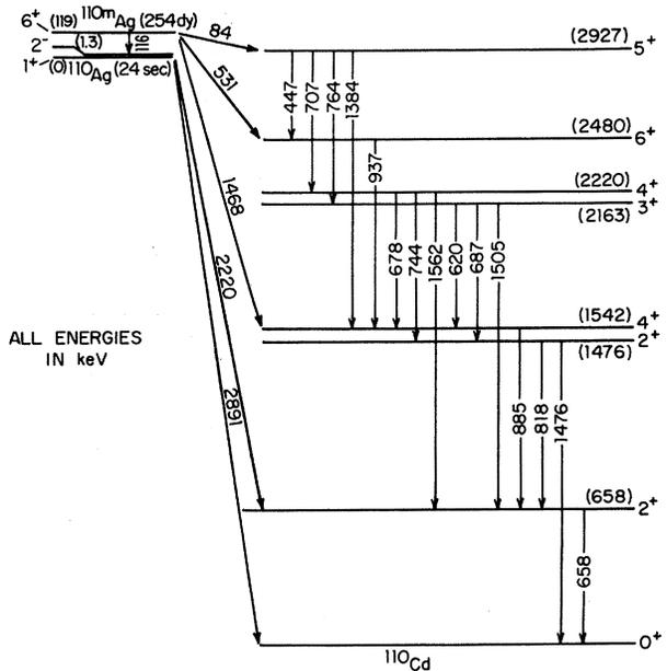
FIG. 2. The energy level diagram for  $^{110m}\text{Ag}$ .
