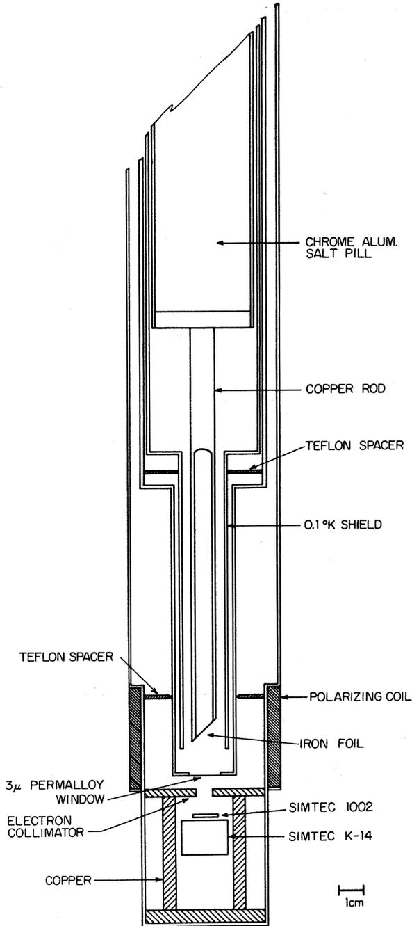
FIG. 1. A diagram of the orientation apparatus showing the relative location of the source, the detectors, the electron collimator, and the polarizing coil.
