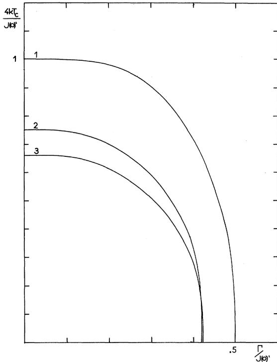
FIG. 1. Phase boundary curve in  $\Gamma$ - $T$  plane for a cubic lattice with nearest-neighbor interactions from (1) molecular field, (2) series expansion, (3) Green's function method.
