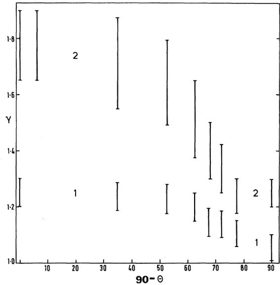
FIG. 2. The critical exponent  $\gamma$  as a function of  $90^\circ - \theta$  for (1) simple cubic and (2) quadratic lattices.
