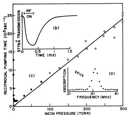
FIG. 1. (a) Tl  ${}^2P_{1/2}$  optical pumping using circularly polarized light, a PAR HR-8 lock-in amplifier, and rf modulation at 1 kHz. The signal peaked for a sidearm temperature of 440°C. (b) Time dependence of the  ${}^2P_{1/2}$  signal with a 5-sec time constant on the waveform eductor. (c) Reciprocal pumping time versus Ne pressure. The cross section is extracted from the slope of the straight line which is a least-squares fit to the open-circle points.
