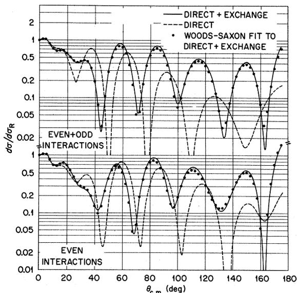
FIG. 1. Differential cross sections for 30-MeV protons on  $^{120}\text{Sn}$ .
