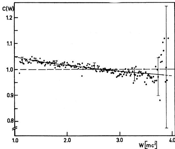
FIG. 1. Spectral shape factor of the  $^{206}\text{Tl} \rightarrow ^{206}\text{Pb} \beta$  transition. The statistical accuracy is below 1% up to  $3mc^2$ . The curve is obtained by fitting the data in the energy range between  $1.38$  and  $3.87mc^2$ .
