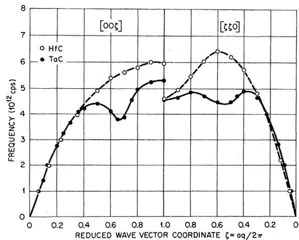
FIG. 2. Longitudinal acoustic modes in Ta and HfC.
