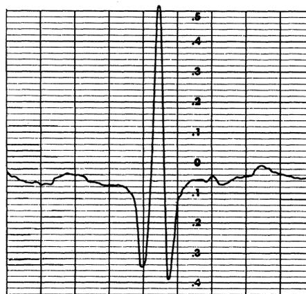
FIG. 2. Recorder tracing of the  $J=0 \rightarrow 1$  rotational transition of DF at 651 099.393 MHz ( $\lambda = 0.46$  mm).
