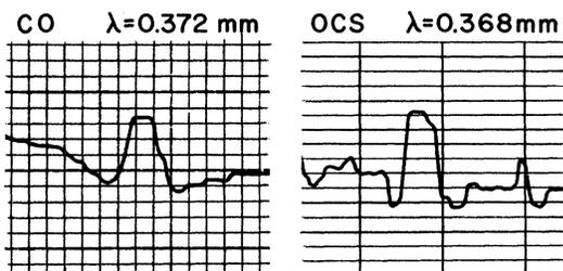
FIG. 1. Recorder tracing of the  $J=6 \rightarrow 7$  rotational transition of CO at 806 651.719 MHz, at left, and of the  $J=66 \rightarrow 67$  transition of OCS at 813 353.706 MHz, at right. Both were observed at the fourteenth harmonic of the klystron frequency.
