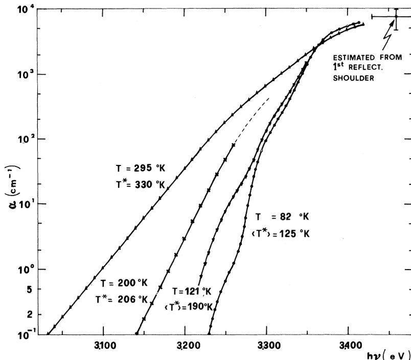
FIG. 1. Absorption coefficient  $\alpha$  of  $\text{SrTiO}_3$  at four different values of temperature  $T$ . For the meaning of  $T^*$  see Eq. (1). A value for  $\alpha$  at 3.46 eV, as roughly estimated from the first shoulder observed in RT reflectance (Ref. 27, see also Ref. 4), is also given.
