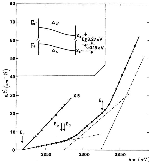
FIG. 2. Square root of absorption coefficient at 121°K versus photon energy. Dots are experimental data; dashed lines are theoretical for indirect edges at  $E_1$ ,  $E_2$ , and  $E_3$ ; and the solid lines are given by their added contributions. The insert shows a schematic picture for the optical gap of  $\text{SrTiO}_3$  in the  $\Delta$  direction.
