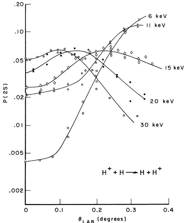
FIG. 1. The measured fractional probability  $P(2s)$  for  $H(2s)$  production in a  $H^+ - H(1s)$  charge-transfer collision, as a function of laboratory scattering angle and laboratory incident proton energy. The uncertainty in the vertical scale is about  $\pm 40\%$ ; the angular resolution is about 0.10 deg full width at half-maximum.
