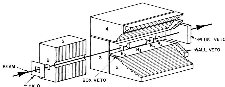
FIG. 1. Counter and spark-chamber assembly. Spark chamber 5 is pulled upstream for clarity.
