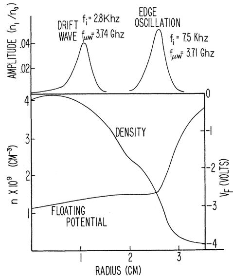
FIG. 2. Demonstration of radial selectivity of excitation of ion resonances through adjustment of incident microwave frequency. The radial positions of excited ion resonances (upper trace) are shown with reference to the density and potential profiles (lower trace).  $f_{ce} = 3.70 \pm 0.005 \text{ GHz}$ .
