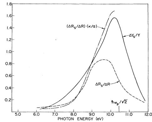
FIG. 3. A comparison of the experimentally determined relative increase in yield,  $\Delta Y_S/Y$ , from a roughened surface of aluminum, with the increase predicted from reflectance measurements on a similarly roughened aluminum surface. The predicted increase in yield is calculated according to a theory which assumes that the decay of excited surface plasmons is the dominant source of additional photoyield.  $Y$  in the above calculation is the smooth-surface photoyield for aluminum.
