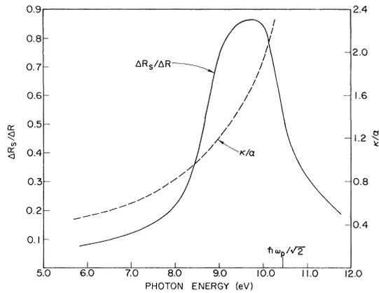
FIG. 2. The experimentally observed relative drop in reflectance,  $\Delta R_S/\Delta R$ , from a roughened surface of aluminum.  $\Delta R_S$ , the difference between the rough- and smooth-surface reflectance, is assumed to result primarily from coupling to surface plasmons.  $\Delta R$  is merely 1 minus the smooth-surface reflectance. Also shown is the ratio of the plasmon energy-decay coefficient  $\kappa$  to the optical absorption coefficient  $\alpha$ .
