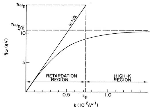
FIG. 1. The surface-plasmon dispersion curve for a free-electron metal having the electronic density of aluminum.  $\omega_p$  is the volume plasma frequency.
