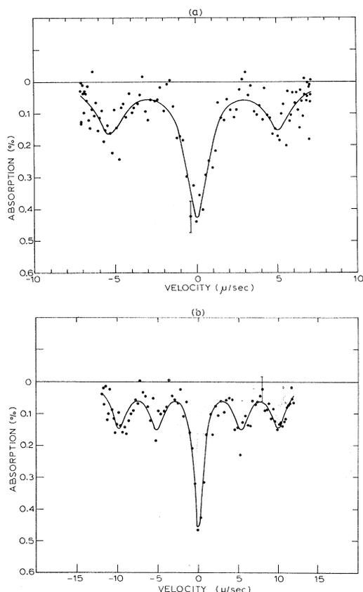
FIG. 1.  $\text{Zn}^{67}\text{O}$  Mössbauer spectra for two velocity ranges: (a) from  $-7$  to  $+7$   $\mu/\text{sec}$ , (b) from  $-12$  to  $+12$   $\mu/\text{sec}$ . Source: 70-h  $\text{Ga}^{67}$  activity produced in  $\text{Zn}^{66}\text{O}$  by  $(d,n)$  reaction. Absorber:  $2.11\text{-g}/\text{cm}^2$   $\text{Zn}^{67}\text{O}$  enriched to 89.6%.
