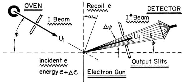
FIG. 1. Experimental schematic. A beam of ground-state particles  $I$  effuses from an oven and is incident at  $\angle\varphi$  on a beam of electrons. The electron impact excites metastable  $I^*$  particles which exit toward a detector in the shape of a "cone"  $(\psi, \Delta\psi)$ . Generally, the angles  $\varphi$  and  $\psi$  are adjusted so as to provide a maximum  $I^*$  signal.
